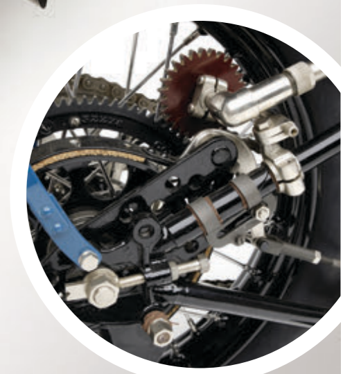
It's hard to miss the speedo drive and rear brake assembly!
