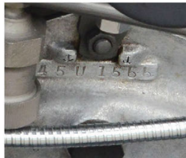
The engine number designates a 1945 U model. The two small anchors above signify US Navy production.
